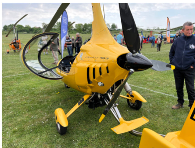
The additional cooling vents, large exhaust muffler, and huge Woodcomp prop are the only obvious external visual differences between a standard Calidus and the Rotax 916 version.
