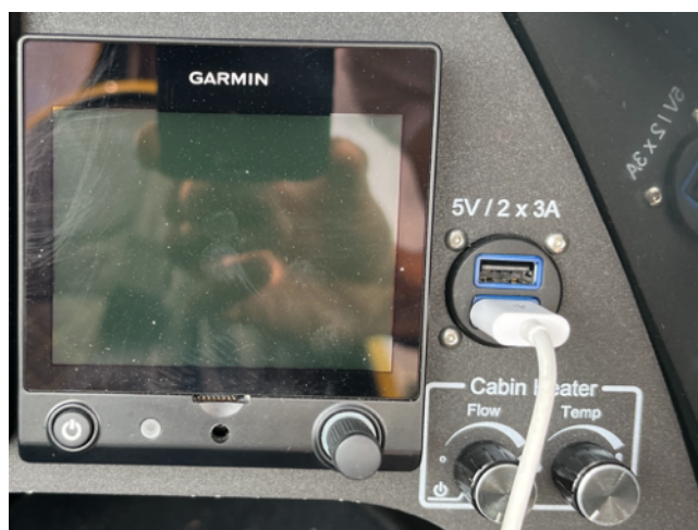
Note the new heater controls to the right of the Garmin G5. You now have fan speed and temperature.
