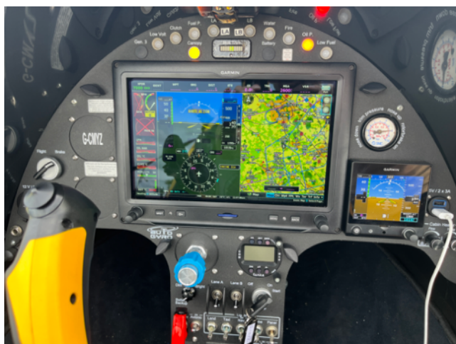
The Garmin G3x is your main display in the centre, the smaller G5 off to the right is your backup auxiliary. You can spec the Calidus to have just the G5 to act as ASI, Altimeter and VSI.
