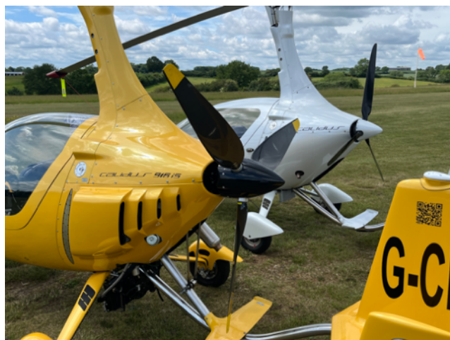
Note the vented bulge, huge prop and spinner when compared with the 914 Calidus in the background.
