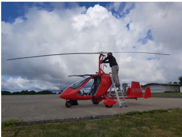
Regreasing the bendix
